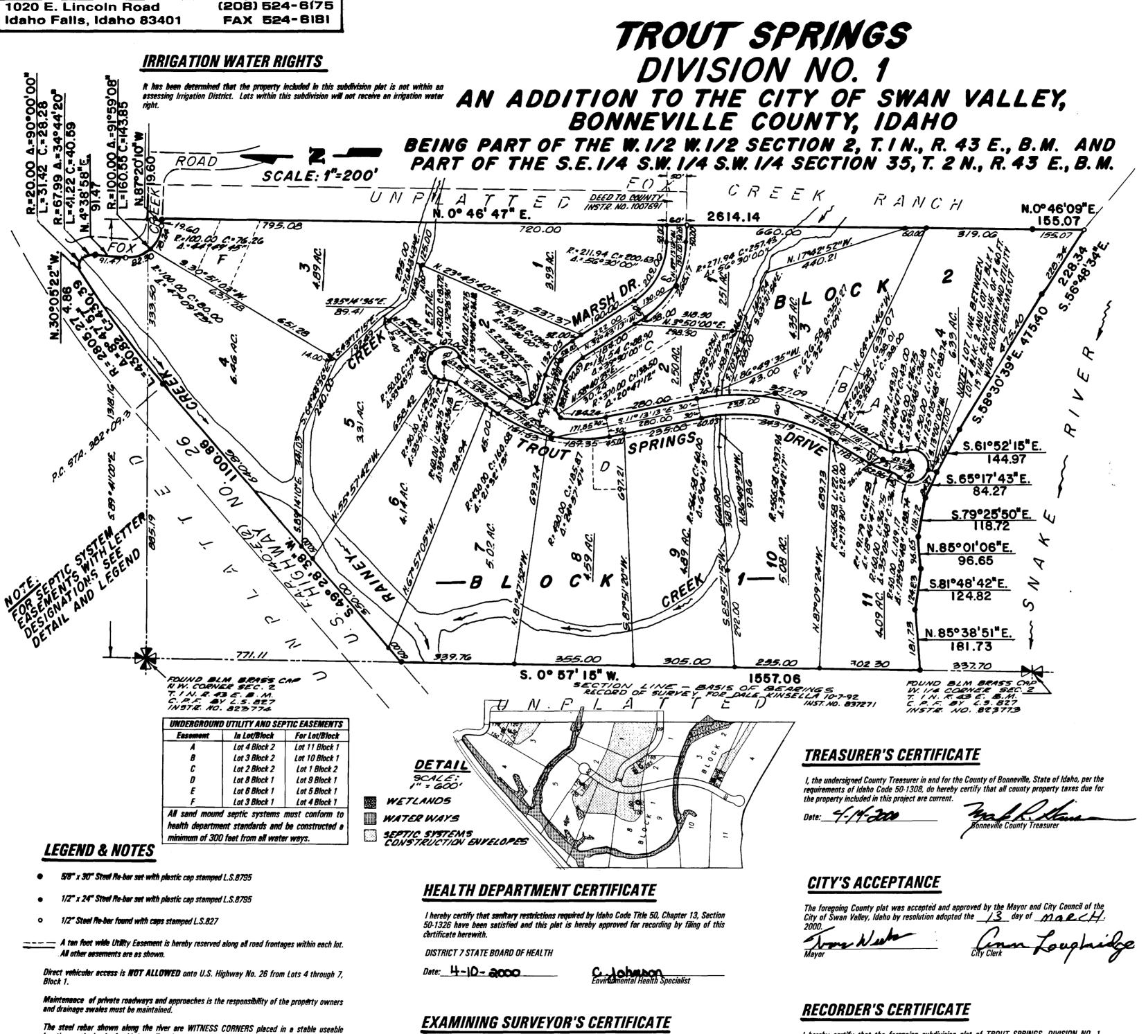
The steel rebar shown along the river are WITNESS CORNERS placed in a stable useable location on the bank of said river. True lot corners are at the mean high water line of the river on an extension of the side lot lines through said witness corners. Bearings and distances shown along the river are traverse lines.
